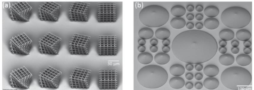
Fig. 1 Special scaffold structures (a) and set of differently shaped microlenses generated using high-precision 3D printing (b).
