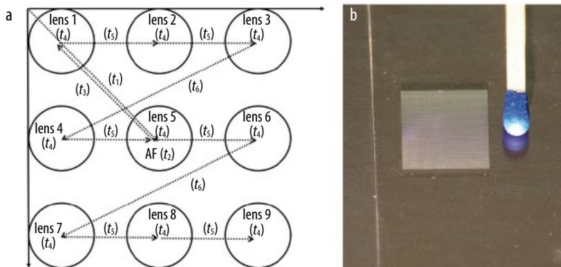
Fig. 4 Unit cell of (3  $\times$  3) microlenses with one single autofocus procedure in the center (a). 1  $\text{cm}^2$  microlens array with a filling factor of 50 % (b).
