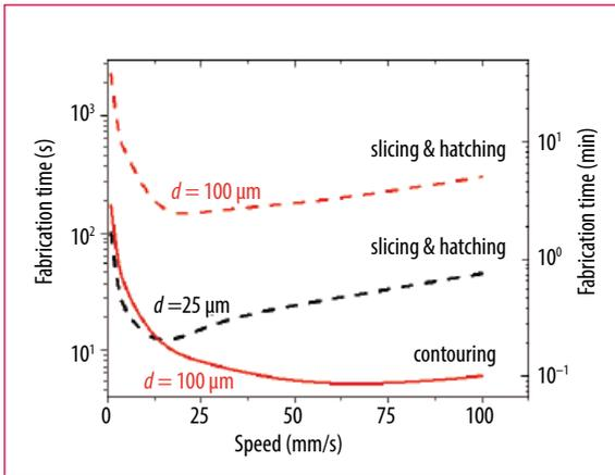
Fig. 3 Comparison of the fabrication times for slicing and hatching of the full volume of microlenses and contouring using circular slices of model microlenses of 25 and 100  $\mu\text{m}$  diameter, respectively.
