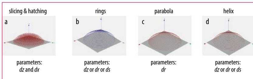
Fig. 2 Exposure strategies to fabricate microlenses. Slicing and hatching typically used by scientists (a), combination of contouring via TPA and UV flash using various strategies (circle, parabola, and helical path, b-d).
